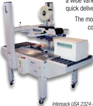
Intertape USA 2324-BB (Bottom Belt Drive) Case Sealer equipped with standard HSD 2000-ET II tape head.
